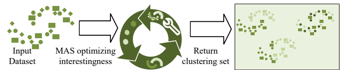
Fig. 2: A short overview of the MAS paradigm. A dataset is input to an optimizer loop finding a good solution for the MAS problem, using HPO. The resulting clustering set is returned to the user.
